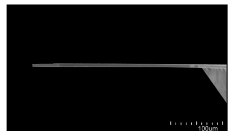
Side view of a PRSA-L300 cantilever
