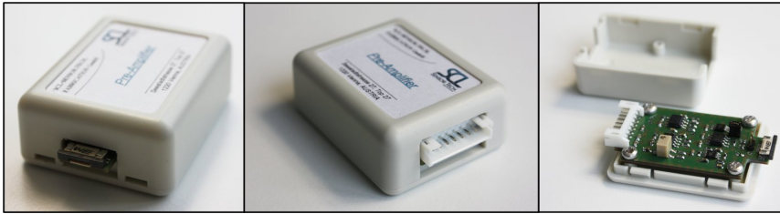
SCL's pre-amplifier (printed circuit board [PCB], connectors and protection case)
