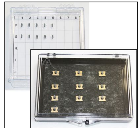
10 self-sensing cantilevers (on PCB or optional as Si-chips), Si-chip h=0.3 mm
